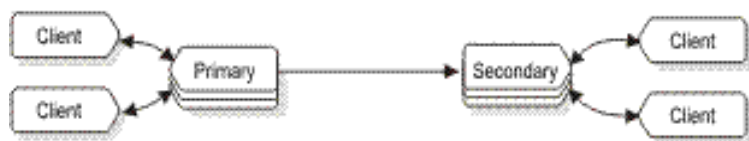
Figure 54. A primary and secondary database server in a data replication configuration
