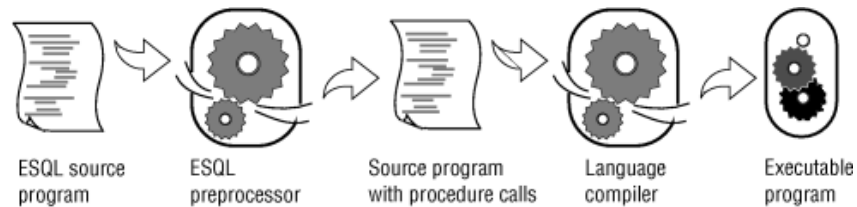
Figure 380. Overview of processing a program with embedded SQL statements
