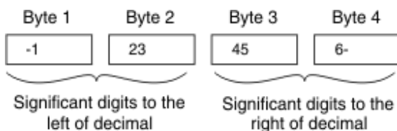
Figure 16. Schematic that illustrates the storage of digits in a decimal (p,s) value
