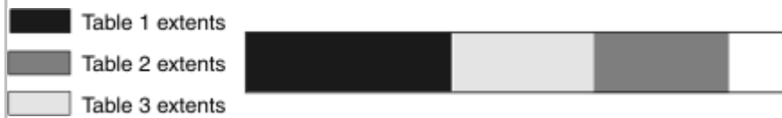
Figure 24. A dbspace reorganized to eliminate interleaved extents
