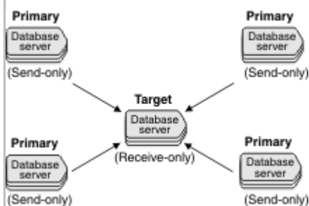
Figure 7. Data Consolidation in a Primary-Target Replication System
