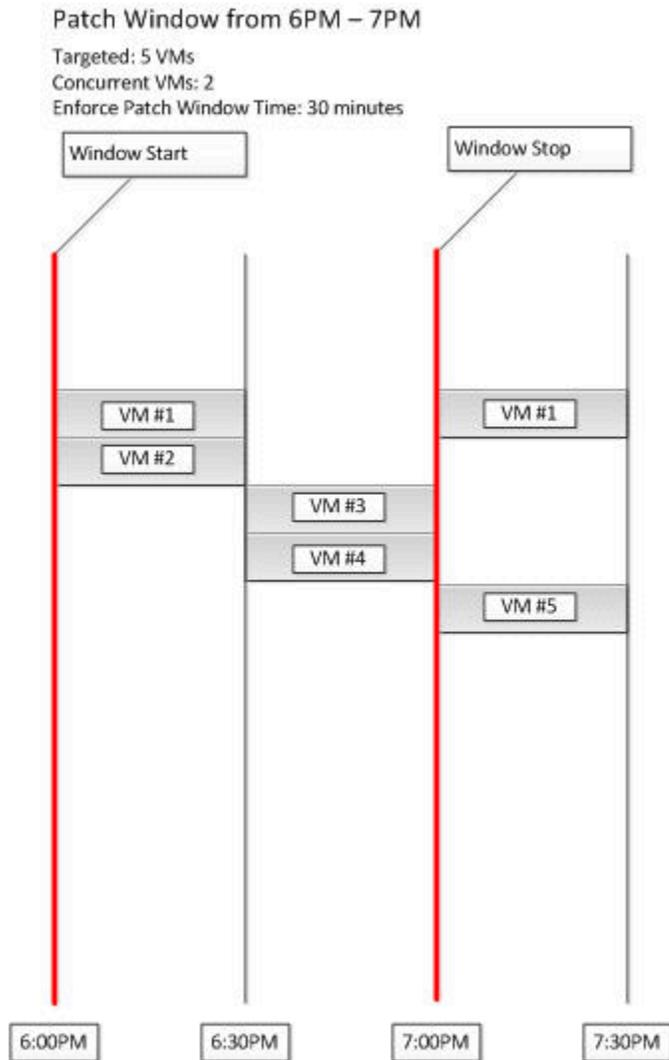
In this example shown in the image, at the beginning of the window, VM#1 and VM#2 starts up. After 30 minutes of being on, VM#1 and VM#2 turns off and #3 and #4 starts. After #3 and #4 turn off, if it's still before 7:00 p.m., VM#5 and VM#1 will start back on again. After 7:00 p.m., no new machines are turned on through this patch window, so when VM#1 and VM #5 turn off at the end of the 30 minute patch window, they won't turn on again.
