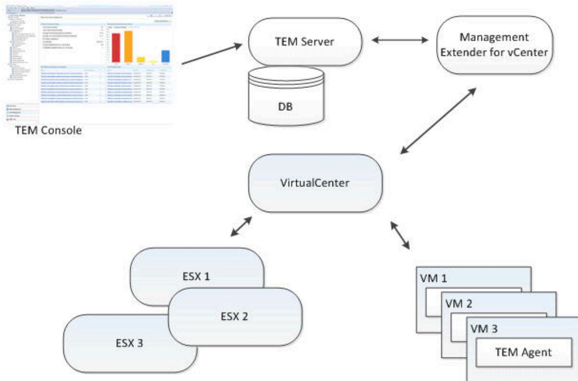
Virtual Endpoint Manager uses the standard BigFix architecture and a management extender.
