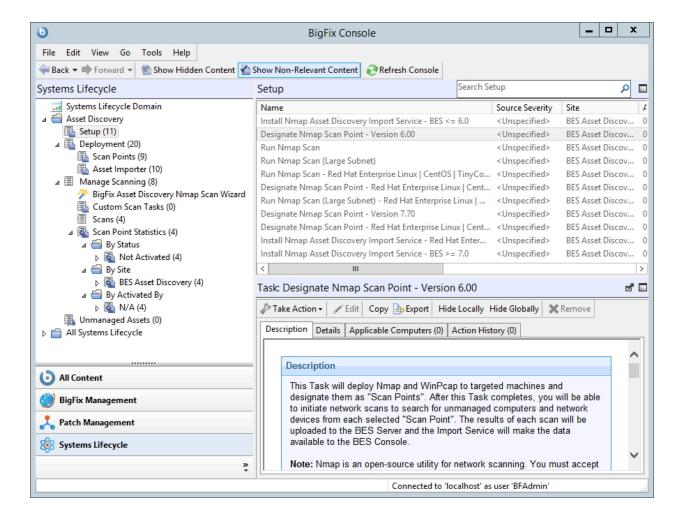
The computers you designate as Scan Points must be running Windows or Linux. These Scan Points are the hubs from which the local subnet is scanned.
