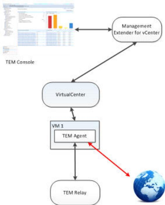
A separate VLAN can be setup and used in conjunction with the offline patch window dashboard. In this setup, the offline virtual machines are switched from a normal network to a VLAN where they can only communicate to a pre-configured BigFix relay. In this setup, the relay can communicate to all of the clients and to the world, but the individual clients cannot communicate with the world.
